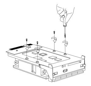
9. Install the drive tray into the backplane board.
